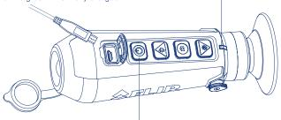
**Turning On/Off** – Press the power button to turn on your OCEAN SCOUT -TK. The Indicator LED is illuminated when power is applied. The FLIR logo is displayed in the eyepiece followed by the live image. To turn OFF press and HOLD the power button. The camera shuts off after one second.
